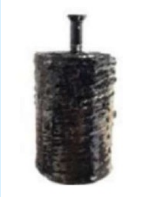
Crude oil remaining on the test piece
