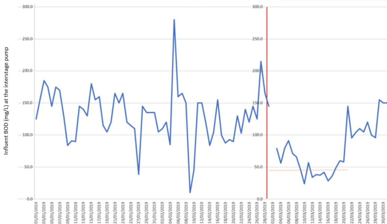
Figure 3: Biological oxygen demand (in mg/L) of the influent wastewater to the plant after the dosing point, before and during the study period. The commencement of BOC dosing is indicated by a vertical red line.
