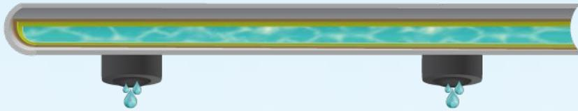
Organic and mineral components within the irrigation water feed the formation of bacteria and mineral fouling of irrigation emitters. These organic components also form the molecular glue which holds inorganic mineral elements together and result in substantial fouling problems in emitters.
