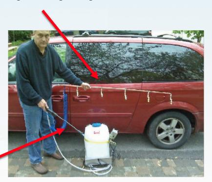
Spray wand is used to spray BOC solution onto garbage spills on the pavement.
