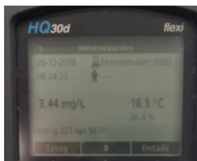
Before Phyto-C 3 TM injection Time 9:24am Dissolved Oxygen 3.4 mg/l Oxygen% 36.4% Temperature 18.5 C
