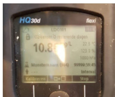
Sustained reading at end of drip line Dissolved Oxygen 10.8 mg/l Oxygen % 123.3% Temperature 21.5 C
