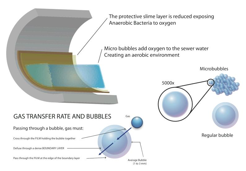
With continuous use of BOC the pipe is cleaned and flow is increased, eliminating the possibility of odor blooms at the same time preventing corrosion
